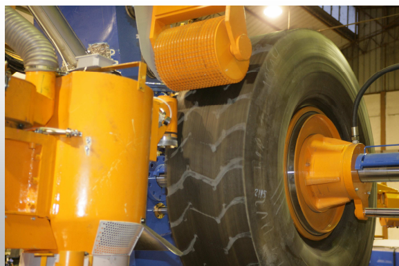
Detail of CNC buffing/peeling head
