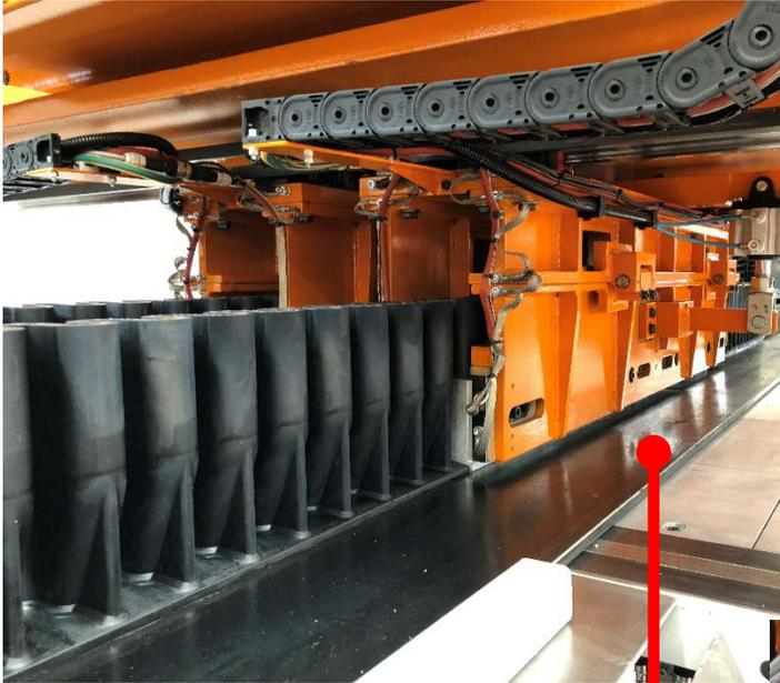
The first station automatically hot-cures the sidewalls onto the base rubber conveyor belt
