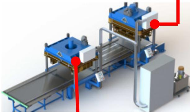
The second station automatically hot-cures the cleats onto the base rubber conveyor belt
